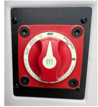
Figure 6-3: Battery Disconnect Switch
