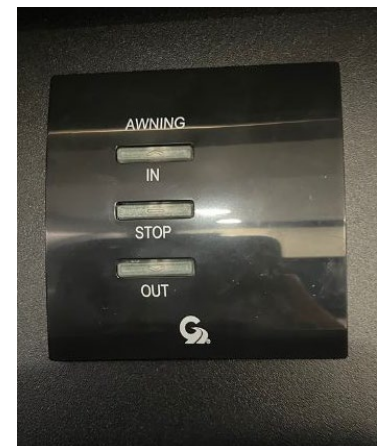
Figure 10-3: Girard Awning Control
