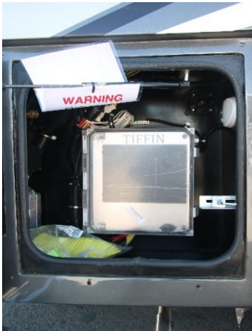
Figure 11-4: M1 Spyder Enclosure located in the driver's side exterior compartment.
