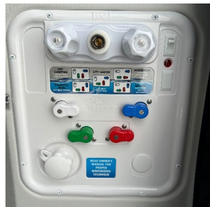
Figure 9-8: Nautilus Sewer Board
