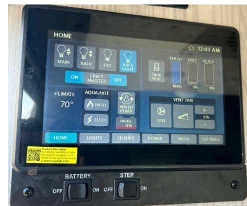
Figure 4-6: Spyder Multiplex Control Panel
