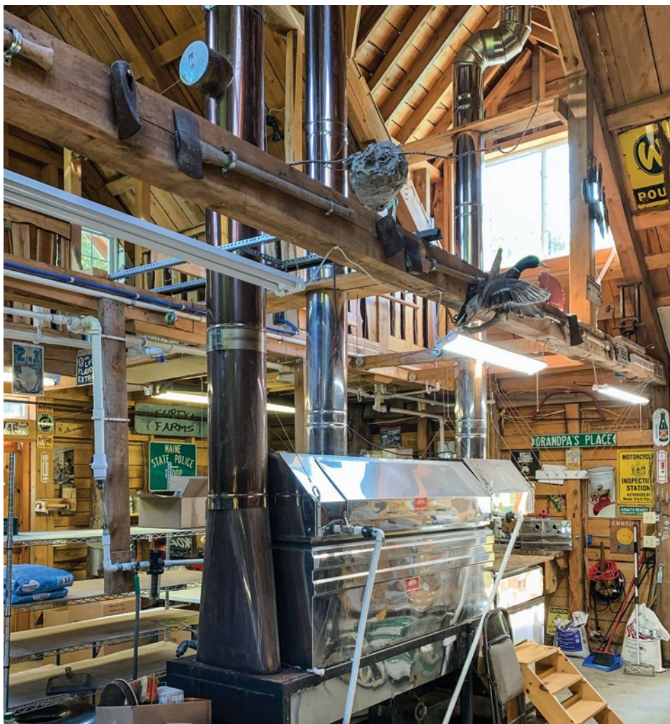
Sap in, syrup out—the wood-fired stainless steel boiler reduces the maple sap to produce the coveted syrup. After a filtering process, the reduction requires 40 gallons of sap to produce one gallon of syrup.
