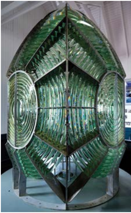
Fresnel lenses, invented in France, bend and concentrate light waves to intensify them. Many lighthouses still use them. They can weigh over 4000 pounds. COURTESY OF WIKIMEDIA
