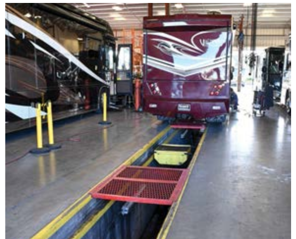
Below left: All fluids for servicing motorhomes are connected by stainless steel lines to bulk tanks on the south end of the service center. Right: One of two service pits allows technicians to take care of engine and transmission oil changes while providing easy access to belts in the engine compartment.
