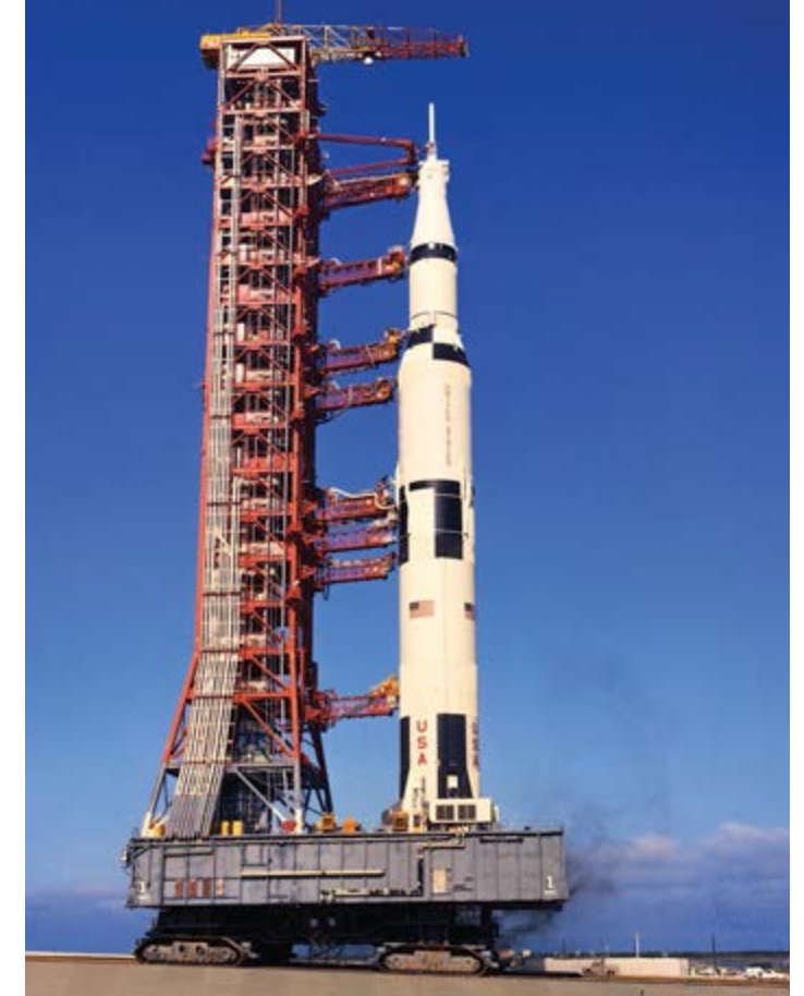
The Missile Crawler Transporter moves the Mobile Launcher Platform carrying the Saturn V rocket and the Apollo capsule to Launch Pad 39A.
