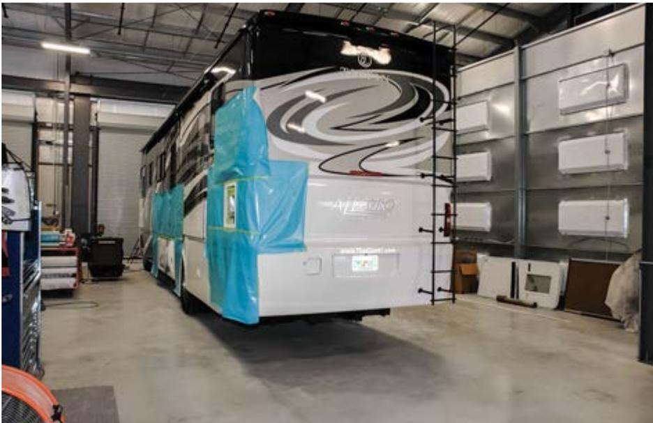
GRW's new service facility boasts 18 bays and offers a fully enclosed paint booth. ♦ Collision and paint specialists can handle a wide array of damages. Here an Allegro Open Road receives taped masking readying it for a short session in the paint booth.
