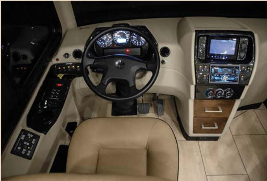
Tiffin included a toggle switch to control the position of the gas and brake pedals. After you have selected the best position for the driver's chair, you can move the pedals in and out to accommodate the height of any driver. The Flexsteel chair has 6-way directional controls and a lever for setting the angle of the back.
