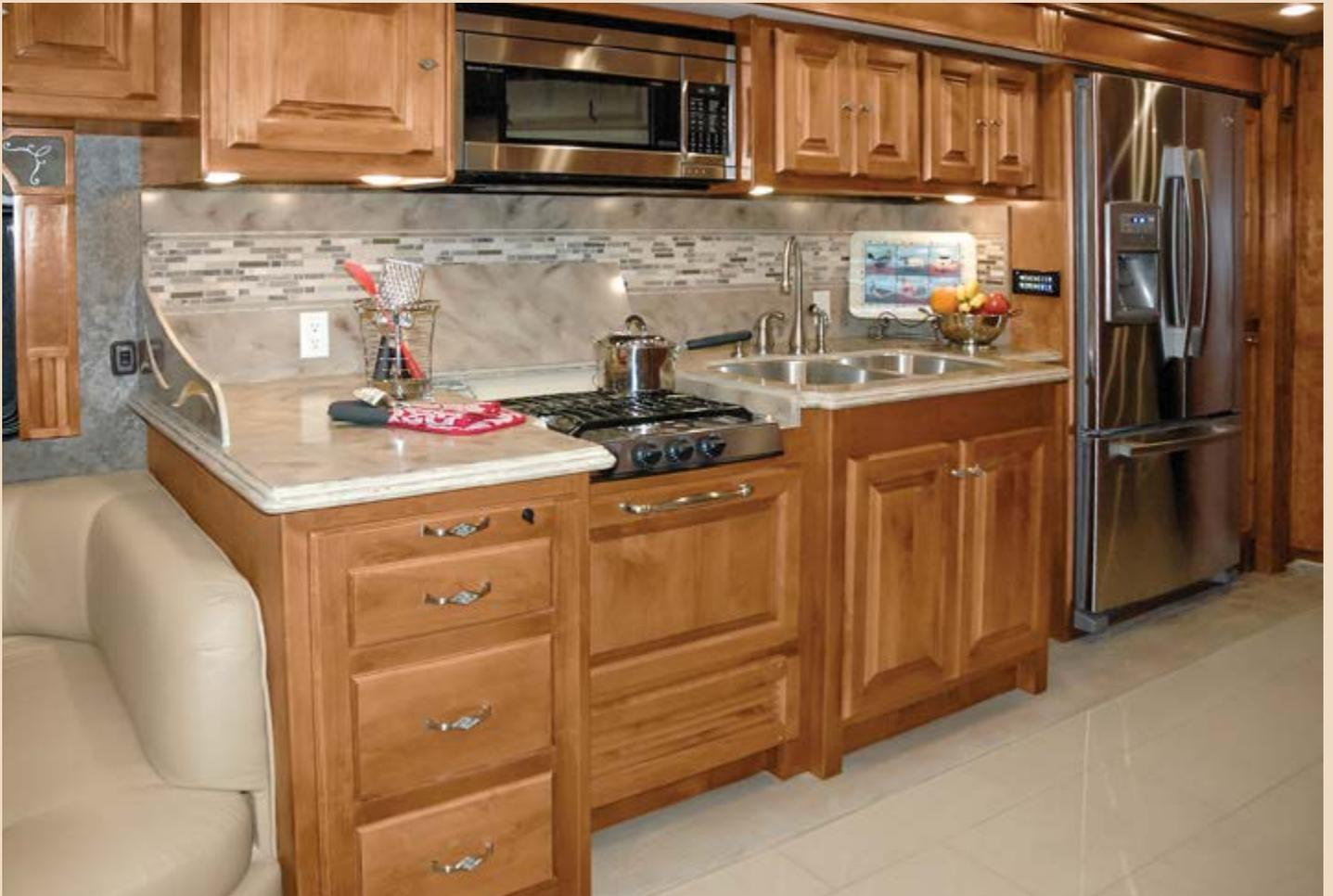
The solid surface counter top is 8 feet wide. The depth varies from 31 to 41 inches. With the Expand-an-Island slide-out deployed, an L-shaped counter top adds another three square feet of work surface or a serving buffet. The slide-out has three drawers.
