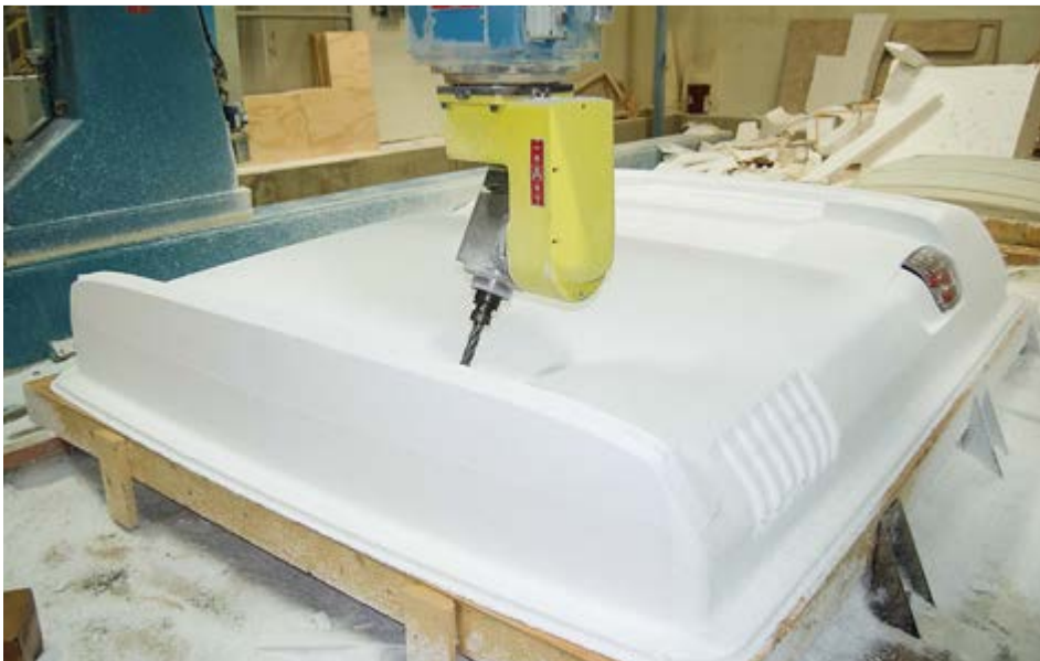
Above: Jeff visits Altec Engineering in Elkhart regularly to check the master forms which they create from his designs. Here, Jeff checks the master form for the fenders on an Allegro Bus. ♦ The data created from Jeff's design was used to program this enormous CNC-router which is carving a rear cap out of polystyrene. This form is cut 3/8-inch deeper than the finished design, and later coated with a self-hardening polyester. The hardened polyester is then recarved to the accurate dimensions. After several finishing processes, it becomes the master male form for creating the female forms which are sprayed with fiberglass to make the rear caps.
