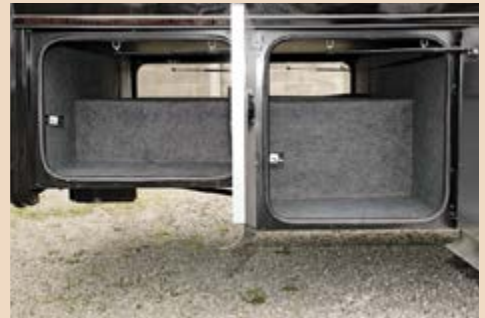
The two rear storage compartments are made of galvanized steel covered with felt, much like the trunk of a car. The pass-through storage design is found in six of the bays
