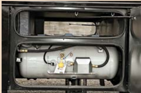
In this mid-section compartment, the propane tank occupies the PS with the generator on the DS. The space above can be used to store your 8-ft. ladder rather than tying it on the back.
