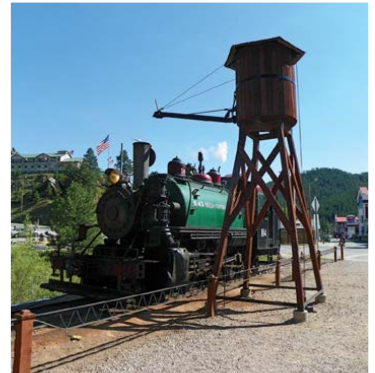
Left: Old Number 110 steam locomotive crosses a highway along its 10-mile route between Hill City and Keystone, South Dakota. Usually pulling six coaches that carry an average of 2,500 passengers every day during the season, the locomotive is 47 feet long, builds steam pressure to 200 PSI, and delivers 37,500 pounds of tractive effort (pulling power). Adults pay $24 for a 20 mile, two hour and 15 minute ride.
