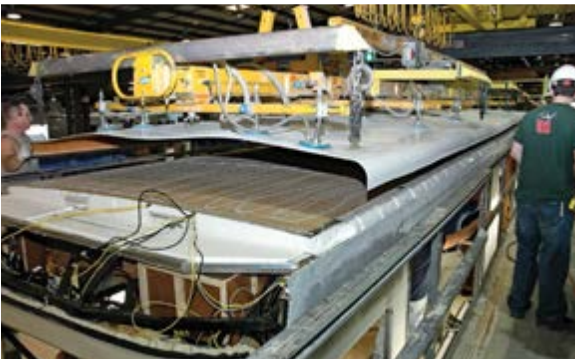
Manufactured in Tiffin's Water Way plant, the one-piece fiberglass roof is glued to the top of the roof assembly.
