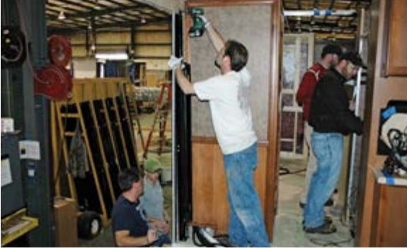
The forward passenger slide-out moves on a vertically mounted power system.
