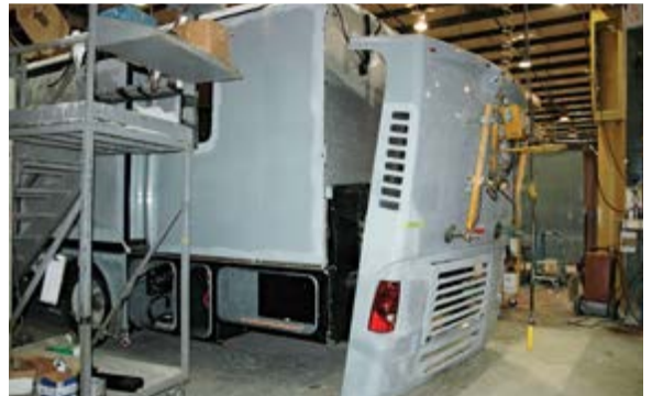
Shown here is the rear cap suspended and ready for installation.
