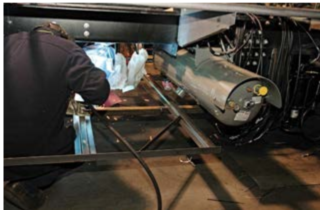
For better balance, the LP tank is turned laterally across the chassis. Note the controls on the rounded end of the tank.
