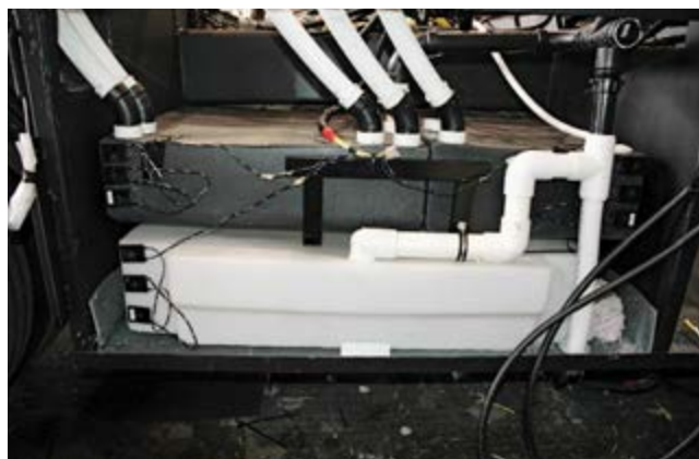
At Station 2 on the assembly line, the white freshwater tank goes in first followed by the grey tank on the left and the black tank on the right.
