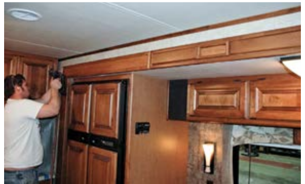
A 4-door gas-electric refrigerator was used in the prototype. Later, in the feature story, you will notice an all-electric residential unit.
