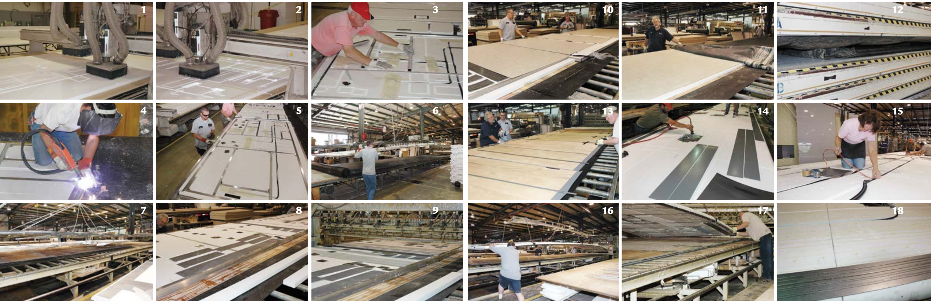
1 Allegro Bay driver's sidewall. At the lower left is the recess or path for a backer plate which will have a wall cabinet attached with screws. 2 Paths for 12-volt and 110-volt wiring. 3 Jimmy Patterson inserts the window assembly studs into a vanity slide-out box. 4 MIG welder Joe Sloan joins studs after insertion into the styrofoam frame. MIG stands for metal and inert gasses. 5 A 42-foot wall with 1 × 1½-inch studs in place is ready for welding. Lewis Cass glues 4 × 4-inch backer plates to exact locations where cabinets will be attached. Wiring in the routed paths awaits lights or electrical outlets. 6 Jason West transfers a
