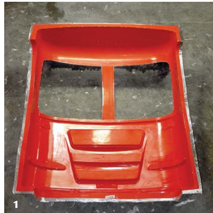
1 This is the mold for the front cap of a 2006 Allegro Bay.
