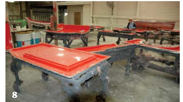
3 After the Gel-Coat, technicians spray a shorter fiberglass to make it have a smoother finish. The spraying device chops the fiberglass strands pulled from a nearby barrel as it is applied and combines it with a resin. 4 After the first fiberglass application has dried, a second application with longer fibers is sprayed into the mold. The longer fibers make the finished fiberglass form much stronger. 5 After the second fiberglass spraying, the form is allowed to cure for two hours before it is de-molded. It takes considerable pressure to pop the fiberglass form from its mold. 6 An empty mold for the shower of a quad-slide Phaeton or Bus awaits an application of Gel-Coat. 7 Shower stalls for a 42-ft. Bus and a 40-ft. Bus that have received Gel-Coat are suspended on the assembly line for a 45-minute drying period. 8 Various molds including a side radiator cover and wheel well covers await Gel-Coat spraying. 9 Larry Mellville removes excess fiberglass and finishes the edges for the shower of an Allegro Bus.
