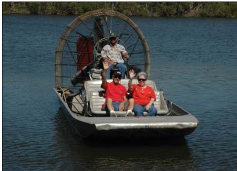
Due to very shallow depths, the air boat is the only practical motor-driven conveyance in the Everglades. Speeds of 45 mph are common.
