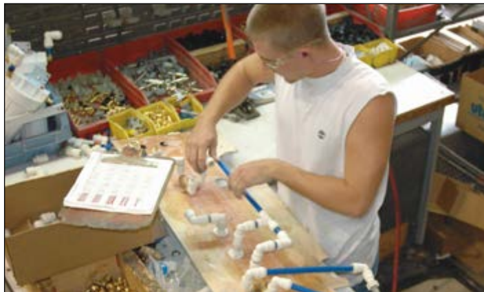
Casey Blanton assembles a water service board at Station 0.
