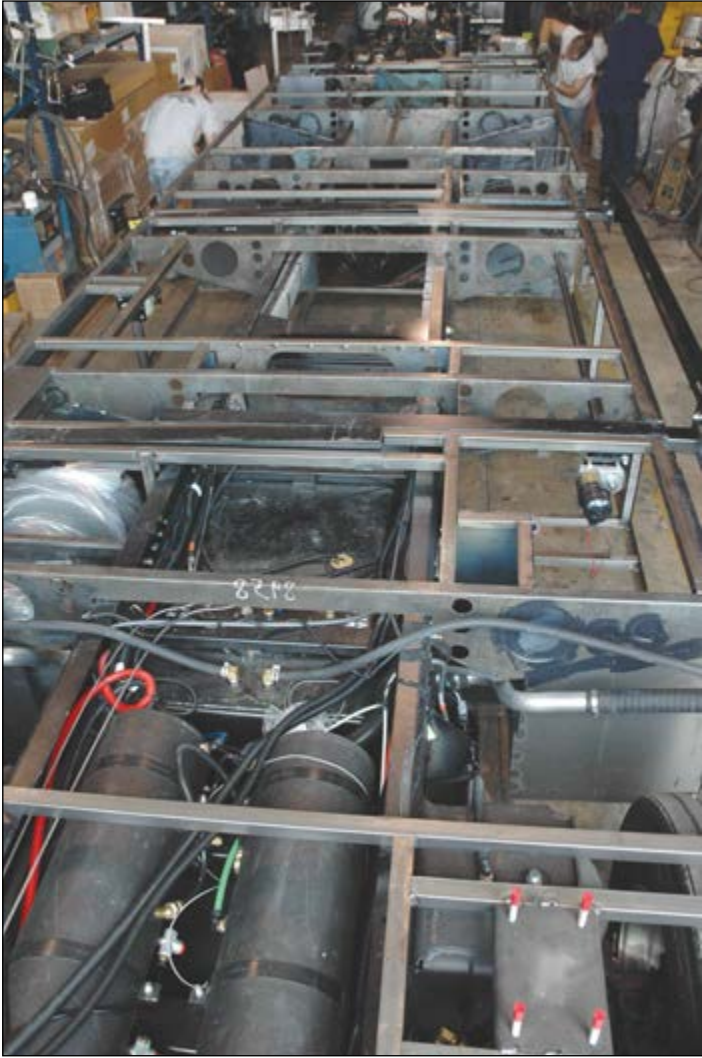
The cross trusses above on this Freightliner chassis provide the additional lateral strength and stability for the larger diesel coaches.
