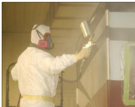
The painters wear white suits for their own protection and to avoid any minute particles from flawing the clearcoat. The clearcoat produces a sparkling gloss finish in all of the colors.
