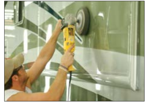
Anthony Searcy buffs the clearcoat finish to create a luster and add a final quality to the full body paint job.
