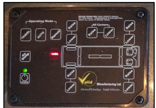
Figure 0-10: Levelling System Control Panel
