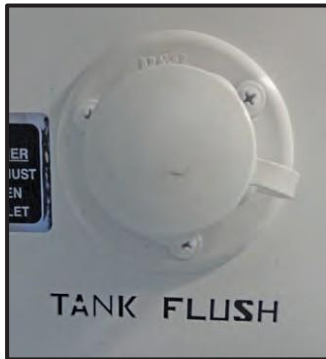
Figure 0-12: Tank Flush Connection
