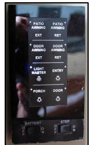
Figure 0-17: 12 VDC Disconnect Switch
