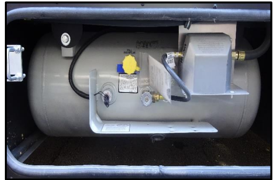
Figure O-2: LP Tank and Regulator
