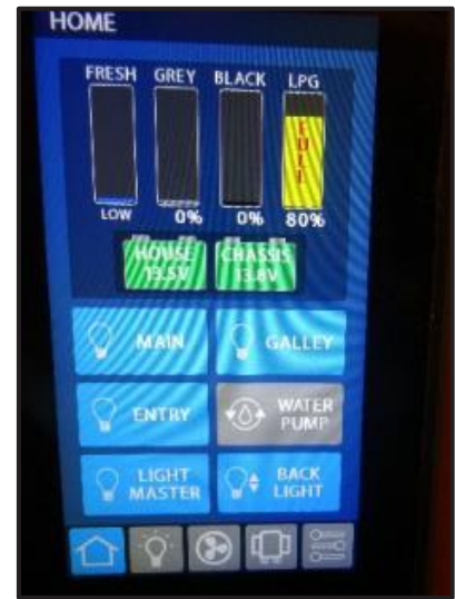
Figure 0-5: Spider Controls System Switch
