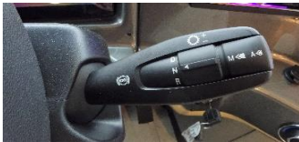
Figure 15-8 Freightliner Transmission Controls
