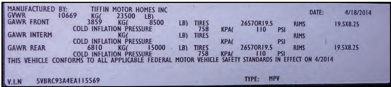
Figure 0-3: Federal Motor Vehicle Standards label located inside the doorway of the coach
