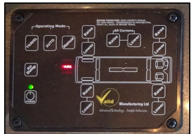
Figure 0-10: Levelling System Control Panel
