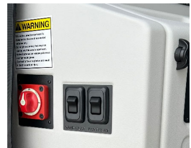
Figure 6-11: Location of Tank and Battery Heat Switches
