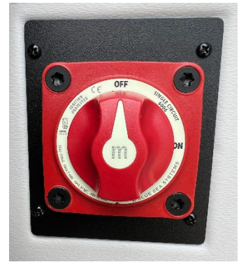
Figure 6-5: Battery Disconnect Switch
