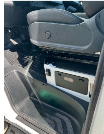
Figure 7-7: Air Compressor Switch Location
