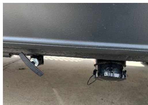
Figure 9-18: Gate Valve and Grey Water Dump Connection
