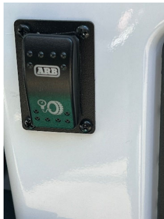
Figure 7-6: Air Compressor Switch
