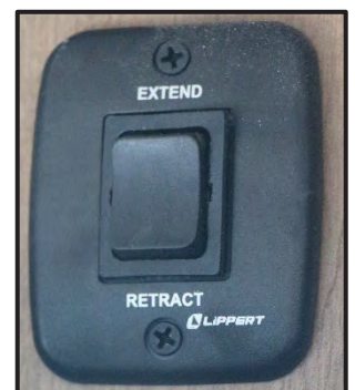
Figure 14-4: Patio Awning Controls
