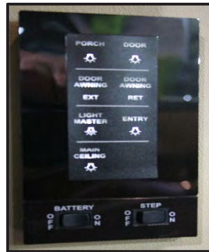
Figure 14-3: Door Awning Controls
