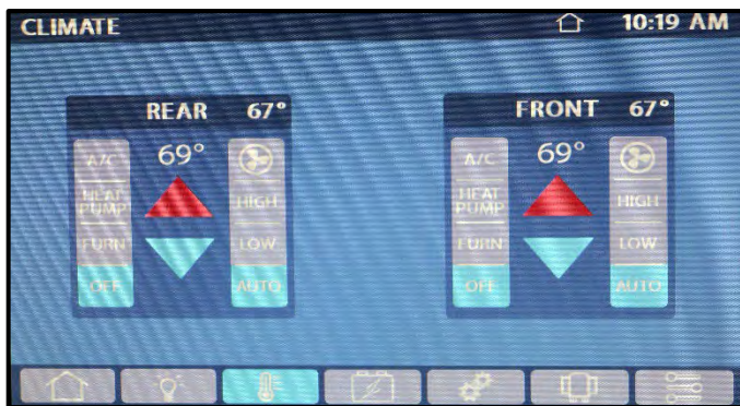
Figure 3-1: Spyder™ Controls System
