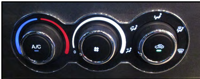
Figure 15-4: Dashboard HVAC Controls
