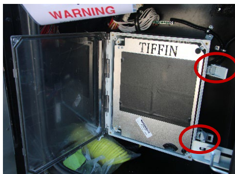
Step 1: Pull latches to open M1 Spyder Enclosure Door.
