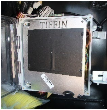
Step 3: With Thumb screws removed, Access M1 Circuit Panel.
