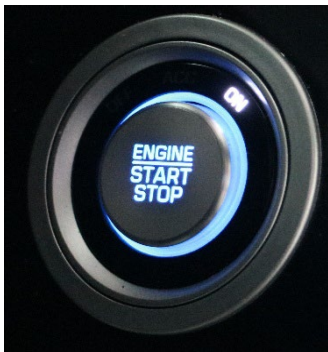
Figure 15-5: Blue Light notifies the driver that the engine is operating.
