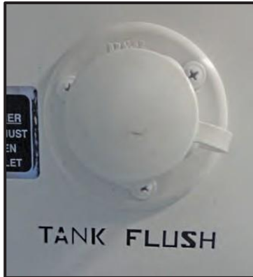
Figure 12-13: No Fuss Flush Connection
