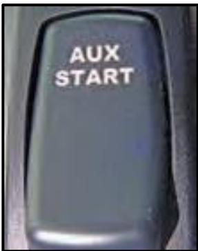
Figure 8-2: Auxiliary Start Switch
