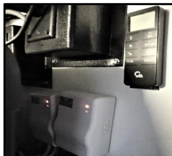
Figure 13-4: Awning Remote Control Module (located in the cargo bay)
