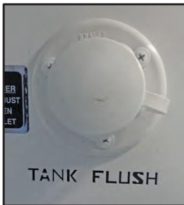
Figure 12-13: No Fuss Flush Connection
