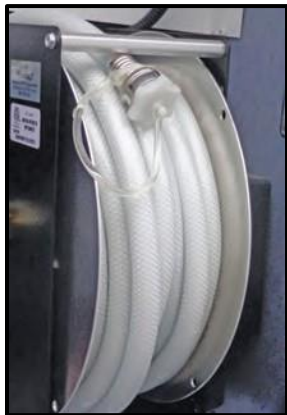
Figure 12-6: Motorhome Water Hose
