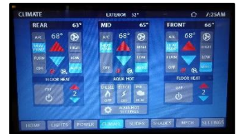
Figure 3-7: Heat Pump Controls
