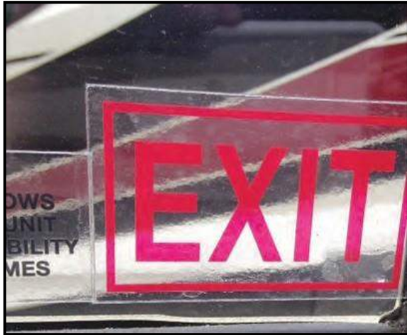
Figure 2-5: Emergency Exit Window
