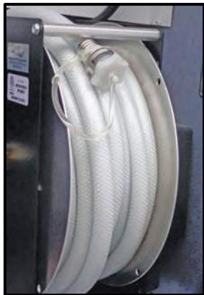
Figure 12-5: Motorhome Water Hose
