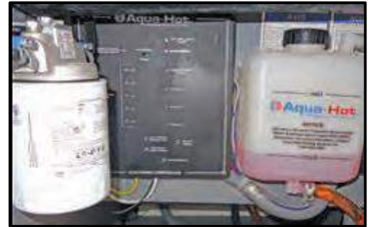
Figure 12-15: Aqua-Hot Surge Tank
