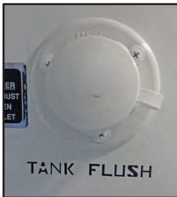
Figure 12-12: No Fuss Flush Connection
