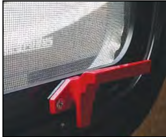
Figure 2-6: Emergency Exit Latch
