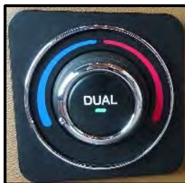
Figure 14-5: Passenger Temperature Control
