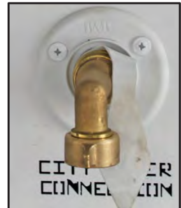
Figure 12-6: City Water Supply Connection
