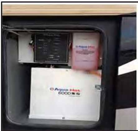
Figure 3-2: Aqua-Hot Surge Tank
