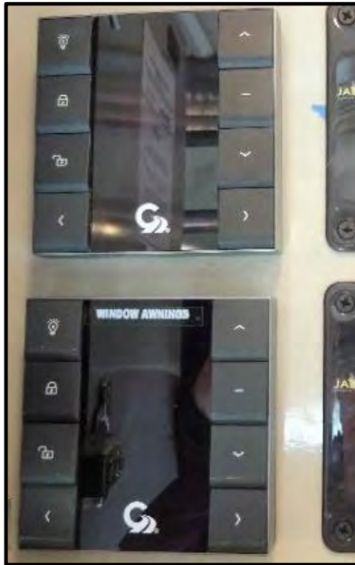
Figure 13-3: Awning Control Switch (in cabinet above driver's seat)
