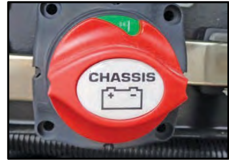
Figure 8-6: Engine Battery Disconnect Panel Switch
