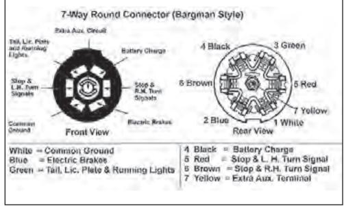
Figure 8-17: Seven-Pin towing connector
