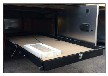
Figure 9-2: Extended Electric Cargo Tray
