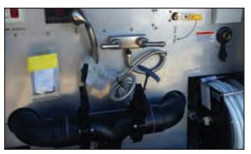
Figure 12-11: Sanitation coupling, valve, and hose
