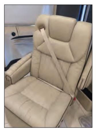
The driver's seat is manually operated and has swivel features. When the motorhome is parked, the driver's seat can be swiveled to face into the living room. To swivel this chair, first extend the slide-out room. Then move the chair backward as far as possible to gain clearance from the steering wheel. Now the chair can be swiveled without interference.
