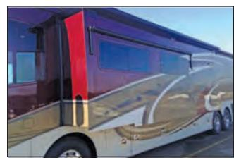
Figure 9-3: Typical slide-out fully extended
