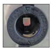
Figure 8-9: 12 VDC receptacle
