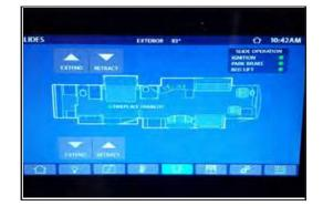
Figure 9-1: Slide-out screen on the Spyder control system
