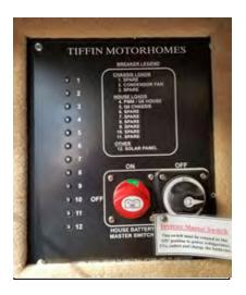
Figure 8-6: 12 VDC disconnect switch
