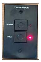
**NOTE:** e booster must be "on" for ANT (a red light will appear) and "off " for the cable (figure 5-4).
