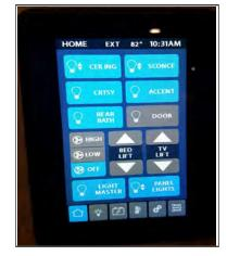
Figure 6-10: Rear Bed Lift on 5" touch Screen
