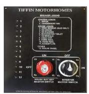
Figure 8-4: House battery disconnect panel switch
