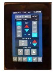
Figure 3-9: A/C Thermostat control page on 5" panel
