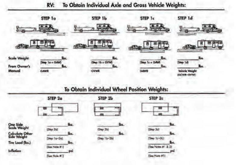
Note 1: From the tire manufacturer's load and inflation tables or the sidewall of the tires mounted on the motor home.
