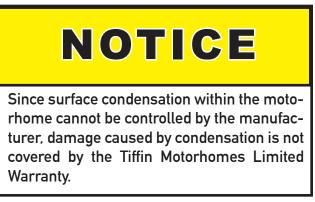
Damage may occur to your vehicle if excessive condensation exists. Accumulation of condensation on surfaces within your motorhome occurs when warm, moist air contacts a cool surface. It is most evident on the inside of windows, but this problem can be controlled by:
