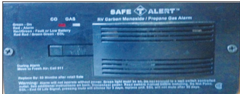
Figure 2-3: Carbon Monoxide alarm
