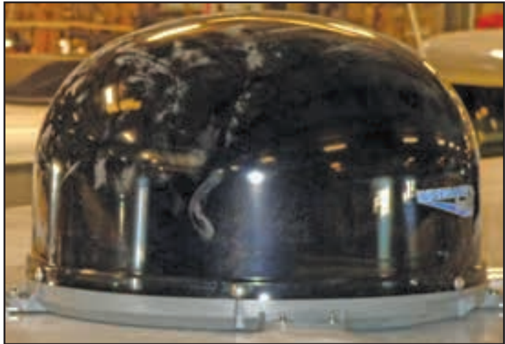
Figure 5-1: The dome satellite on top of the motorhome can be raised allowing easy access to change switches to a new satellite provider.
