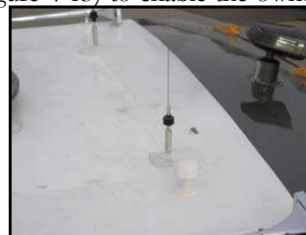
Figure 4-13. CB Antenna Installation
