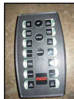
Figure 10-4. Control for Living Area Power Shades
