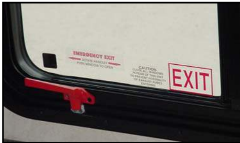
Figure 13-2. Emergency Exit Window
