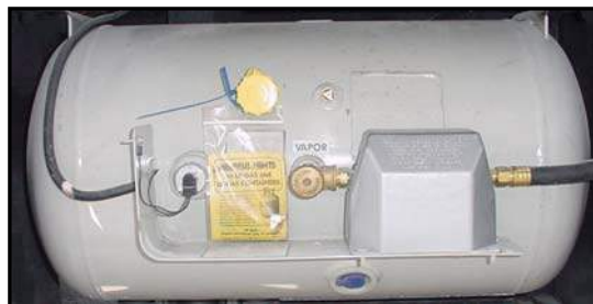
Figure 2-5. Liquid Propane Tank
