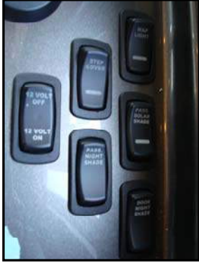
Figure 10-6. Control for Passenger & Entry Door Power Shades
