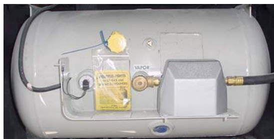
Figure 3-7. Liquid Propane Tank
