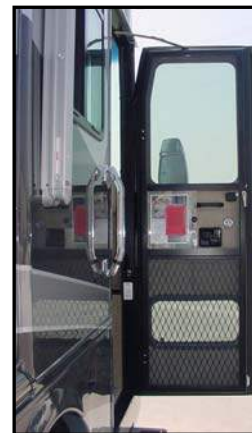
Figure 13-6. Front Door & Screen Door
