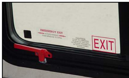
Figure 2-9. Emergency Exit Window
