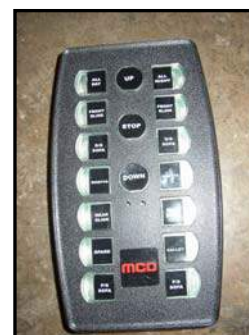
Figure 10-4. Control for Living Area Power Shades
