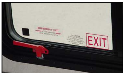
Figure 13-2. Emergency Exit Window
