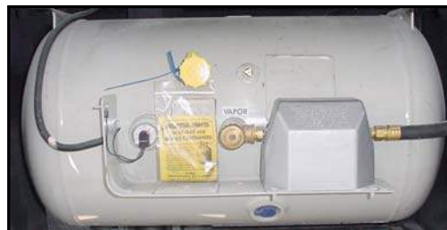
Figure 2-4. Liquid Propane Tank
