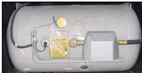
Figure 2-5. Liquid Propane Tank
