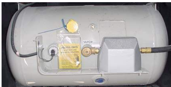
Figure 3-6. Liquid Propane Tank
