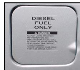
Figure 2-3. Fuel Tank Fill Door
