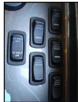
Figure 7-10 12 VDC Disconnect Switch
