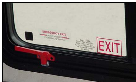
Figure 2-9. Emergency Exit Window
