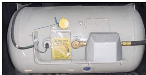
Figure 2-4. Liquid Propane Tank
