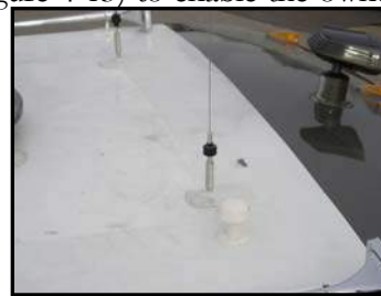
Figure 4-13. CB Antenna Installation
