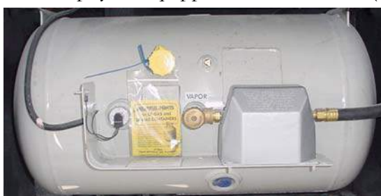
Figure 3-6. Liquid Propane Tank
