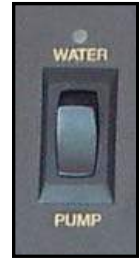
Fig. 11-5. Water Pump Switch
