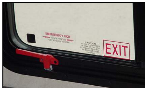
Figure 2-9. Emergency Exit Window
