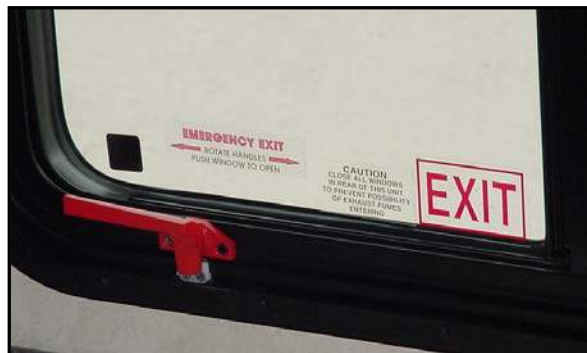
Figure 2-9. Emergency Exit Window
