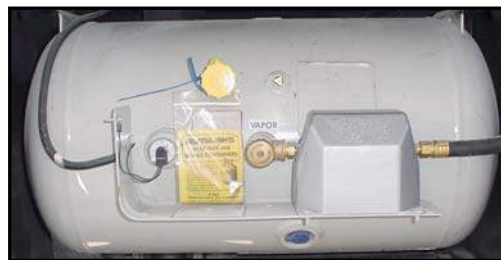
Figure 2-4. Liquid Propane Tank
