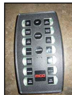
Figure 10-4. Control for Living Area Power Shades
