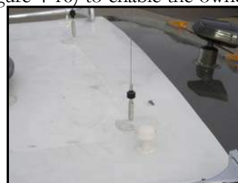
Figure 4-16. CB Antenna Installation
