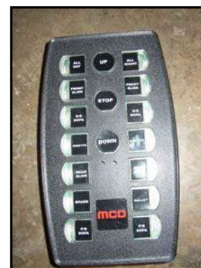
Figure 10-4. Control for Living Area Power Shades
