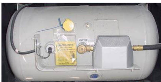
Figure 3-6. Liquid Propane Tank
