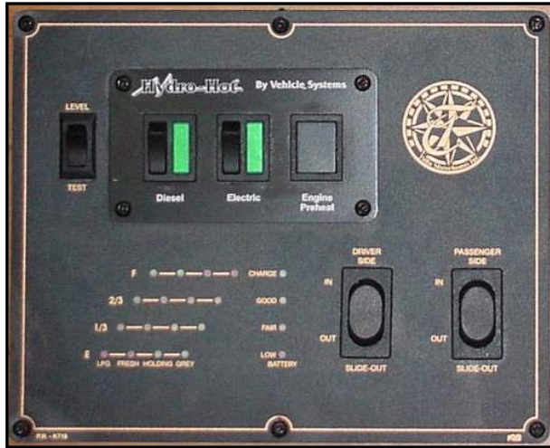
Figure 11-1. Monitor Panel (Water, LP Gas, Battery)
