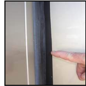
Figure 14-6. Inspecting Slide Out Gasket
