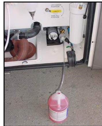
Figure 14-17. Winterizing the Water System
