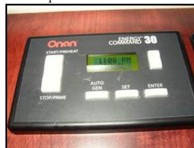
Figure 7-15. Automatic Generator Switch
