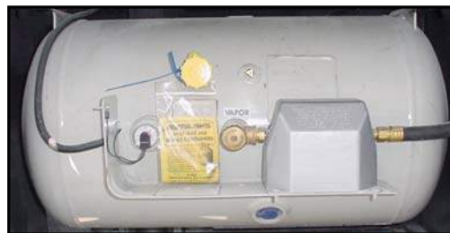
Figure 2-3. Liquid Propane Tank
