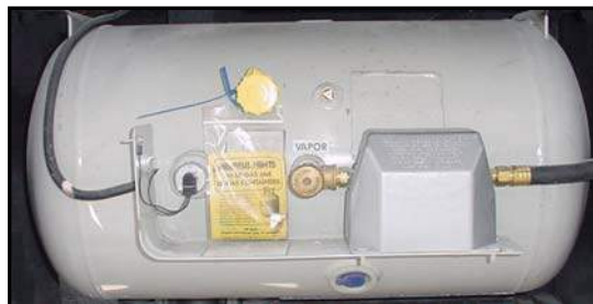
Figure 2-4. Liquid Propane Tank
