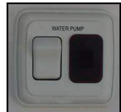
Figure 11-6. Water Pump Switch
