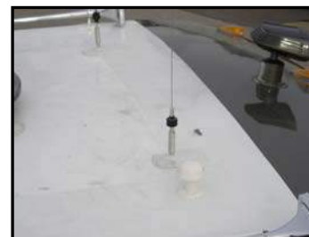
Figure 4-16. CB Antenna Installation
