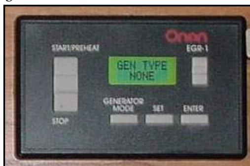
Figure 7-17. Automatic Generator Starting (AGS) System
