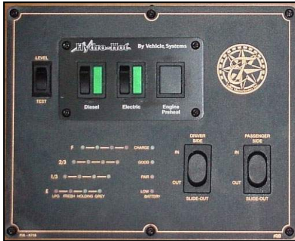
Figure 11-1. Monitor Panel (Water, LP Gas, Battery)
