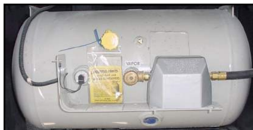
Figure 2-3. Liquid Propane Tank
