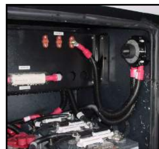
Figure 7-8. Rotary Switch to Disconnect “House” Batteries
