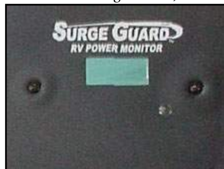
Figure 7-19. Surge Guard Display Panel
