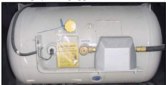
Figure 3-4. Liquid Propane Tank
