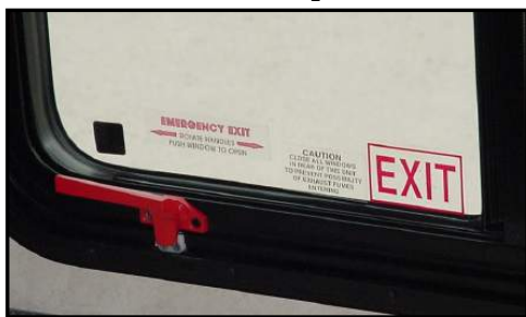
Figure 13-2. Emergency Exit Window
