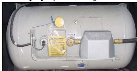
Figure 2-4. Liquid Propane Tank
