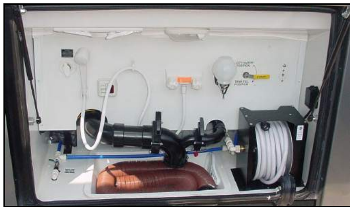
Figure 11-12. Sanitation Compartment Containing Holding Tank Drains and Flexible Drain Hose
