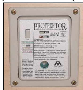
Figure 3-6. LP Gas Detector
