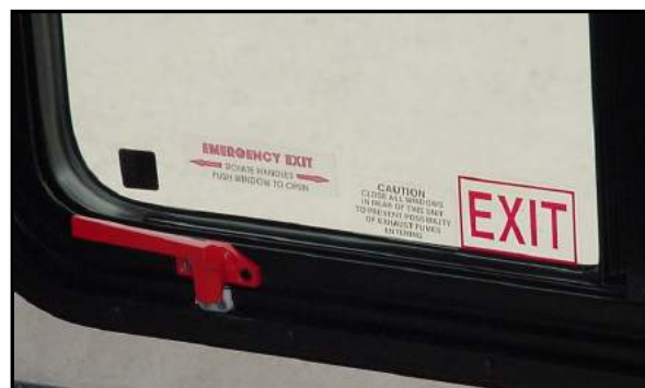
Figure 2-8. Emergency Exit Window
