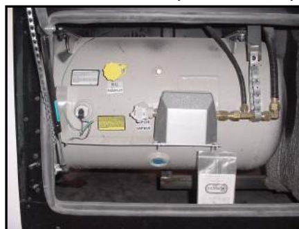
Figure 2-4. Liquid Propane Tank
