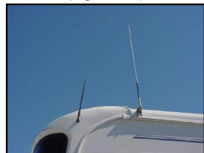
Figure 4-19. CB Antenna Installation
