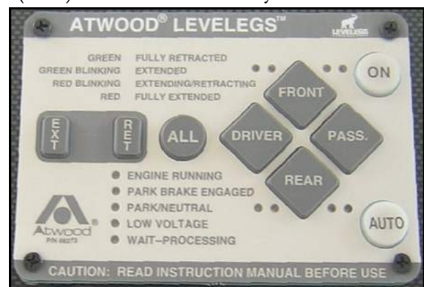
Figure 9-6. Leveling Control Panel on Dashboard
