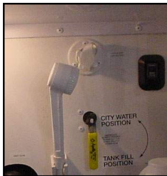
Figure 11-8. City Water Connection
