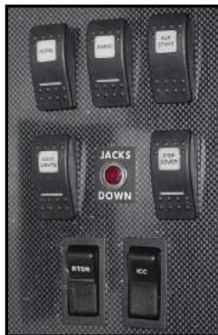
Figure 7-3. Auxiliary Start Switch
