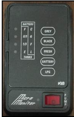
Figure 11-1. Monitor Panel (Water, LP Gas, Battery)
