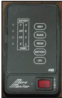
Figure 11-1. Monitor Panel (Water, LP Gas, Battery)
