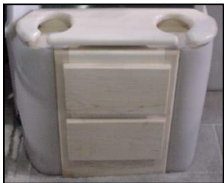
Figure 14-10. Driver's Console Cabinetry
