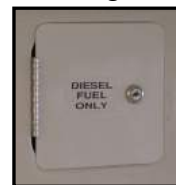
Figure 2-3. Fuel Tank Fill Door
