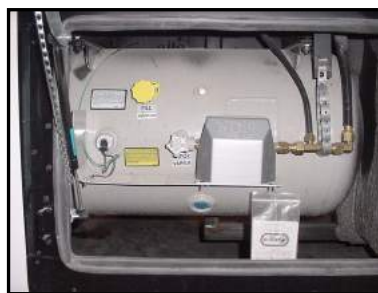
Figure 2-2. Liquid Propane Tank
