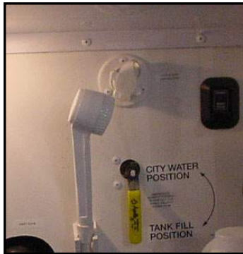
Figure 11-7. City Water Connection
