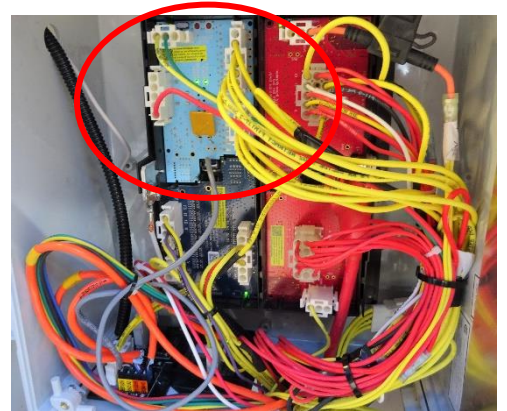
Figure 12-4: Location of Slide-Out Room Control Override behind the front panel.
