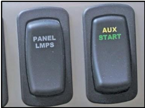
Figure 11-2: Auxiliary Start Switch
