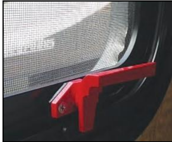
Figure 2-9: Emergency Exit Latch
