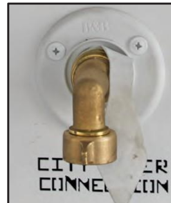
Figure 14-8: City Water Supply Connection
