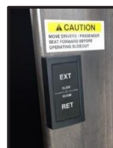
Figure 11-2: Front Slide-Out Switch
