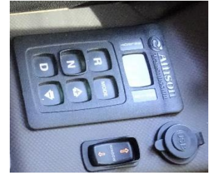
Figure 16-7 PowerGlide Tran Controls
