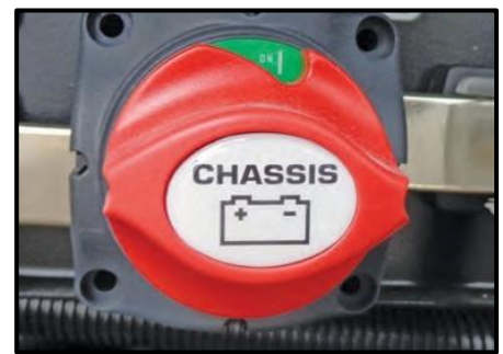
Figure 10-5: Engine Battery Disconnect Switch
