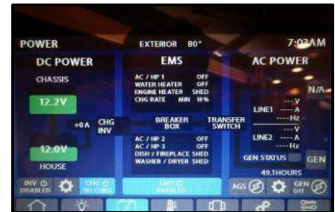
Figure 10-14: Energy Management System
