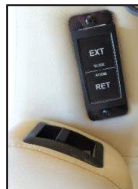
Figure 11-1: Front Slide-Out Switch
