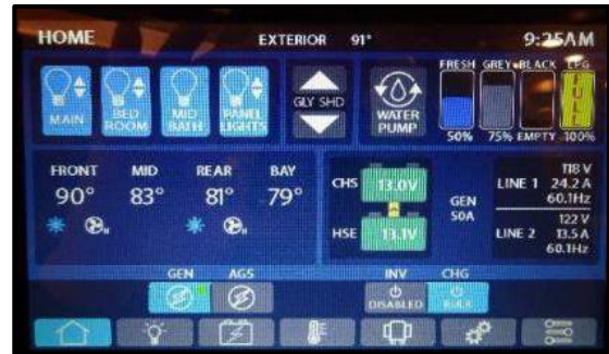
Figure 4-3: Spyder Controls System
