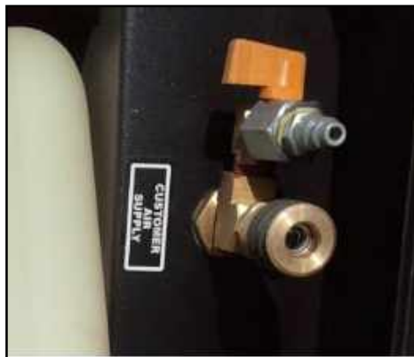
Figure 8-2: Rear Customer Air Supply
