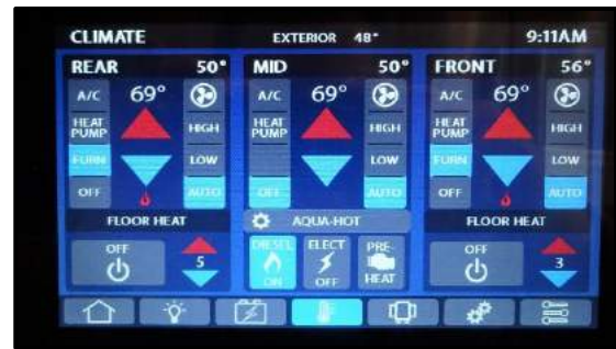
Figure 4-3: Spyder Controls System
