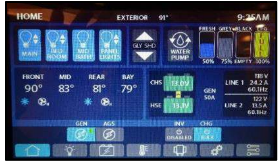
Figure 3-1: Home Screen for the Spyder Controls System
