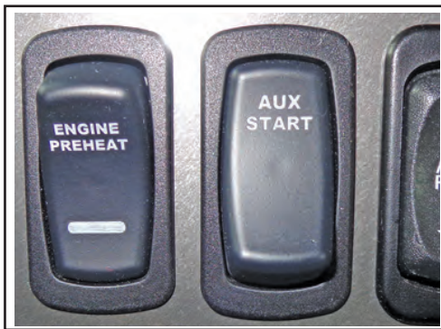
Figure 10-3: Auxiliary start switch
