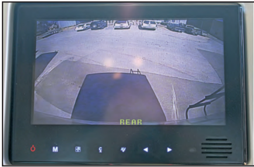
Figure 16-1: Rear-view camera monitor
