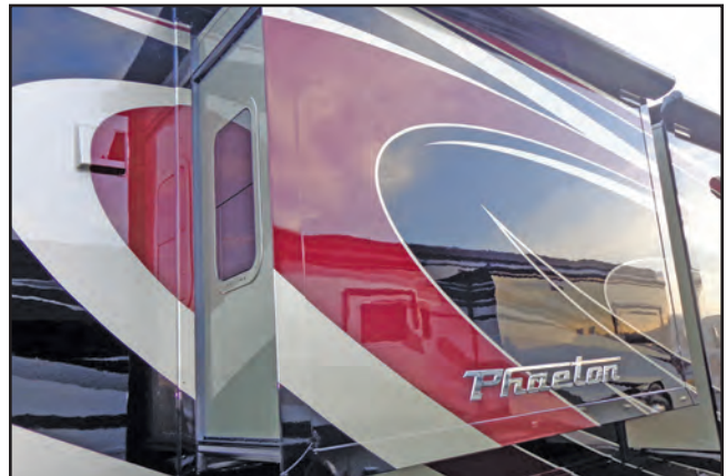
Figure 11-3: Typical slide-out fully extended
