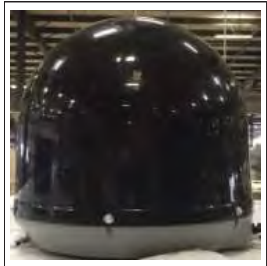
Figure 7-1: The dome satellite located on top of the coach can be raised, allowing easy access to change switches to a new satellite provider.
