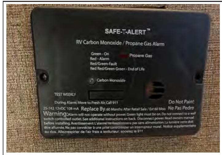
Figure 2-5 Carbon Monoxide Alarm
