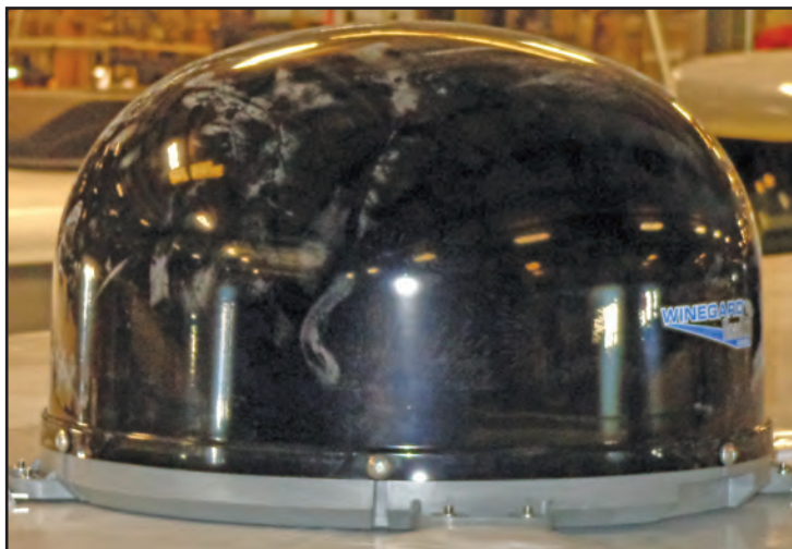
Figure 7-1: The dome satellite on top of the motorhome can be raised allowing easy access to change switches to a new satellite provider.
