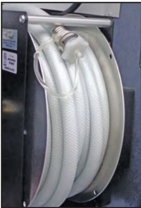
Figure 13-6: City water supply connection
