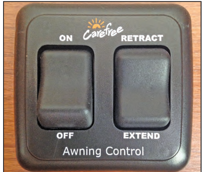
Figure 15-3: Power patio awning control switch located in the cabinet above the driver's side console
