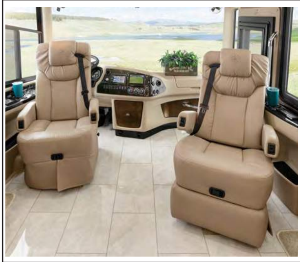
Figure 8-5: Both the driver's and passengers chairs swivel to face the living area of the coach
