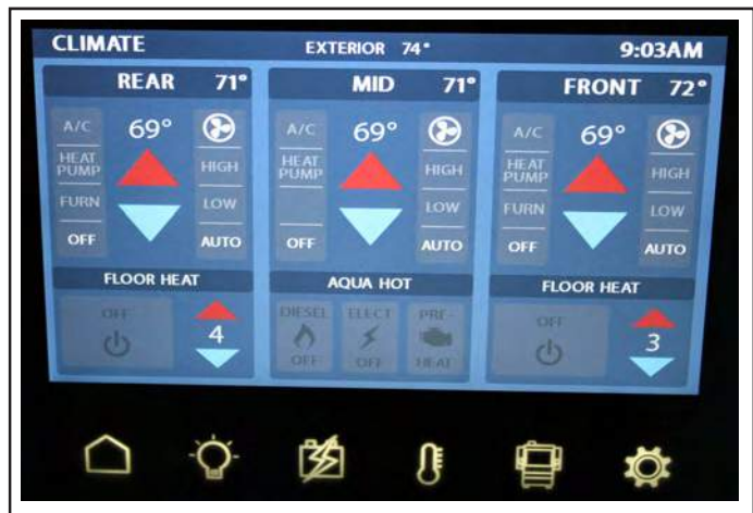
Figure 4-3 Thermostat on Spyder Control System
