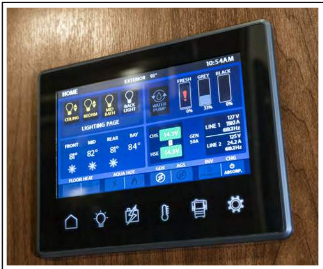
Figure 3-1: Spyder Controls Multiplex System
