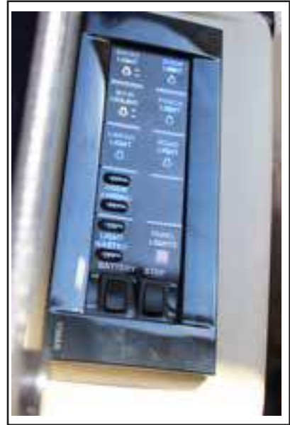
Figure 11-6: Entrance step switch
