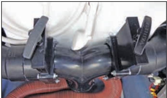
Figure 13-10: Sanitation coupling, valve and hose
