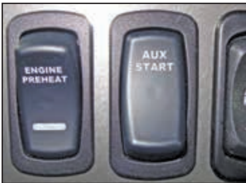
Figure 9-3: Auxiliary start switch
