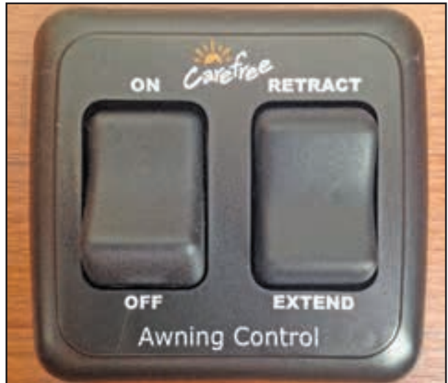
Figure 14-3: Power patio awning control switch located in the cabinet above the driver's side console
