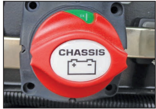
Figure 9-6: Engine battery disconnect panel switch
