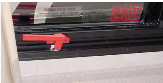
Figure 12-2. Bedroom Emergency Exit Windows
