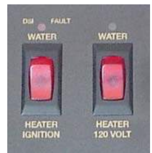
Figure 4-16. Water Heater Switches
